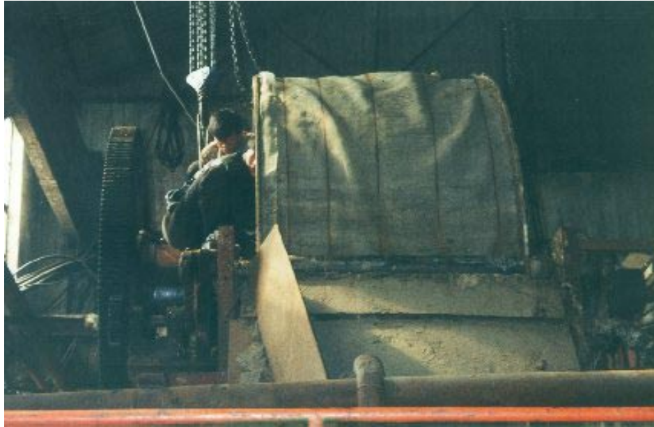
Photo 13: Vacuum straw pulp washing
