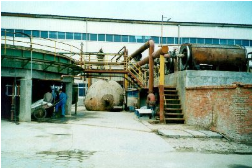
Photo 11: Wastewater treatment rotating screens
