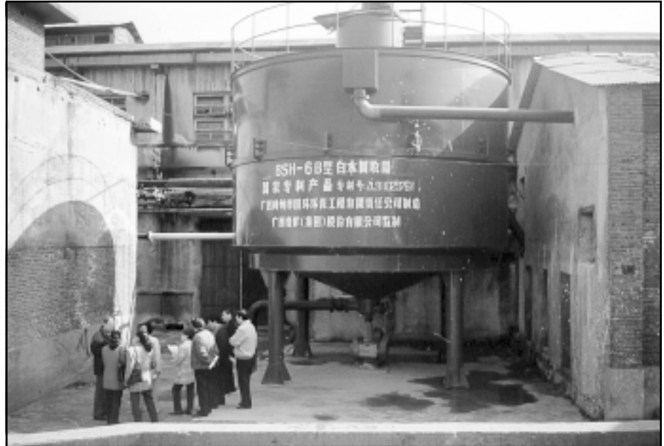
This tank recycles water from two paper machines. The equipment costs 310,000 RMB and reduces COD emissions by 90%, TSS by 94%, and recovers 390,000 RMB worth of fibre per year.
